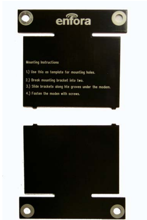
Figure 5 - MT-GL Mounting Bracket (separated)
