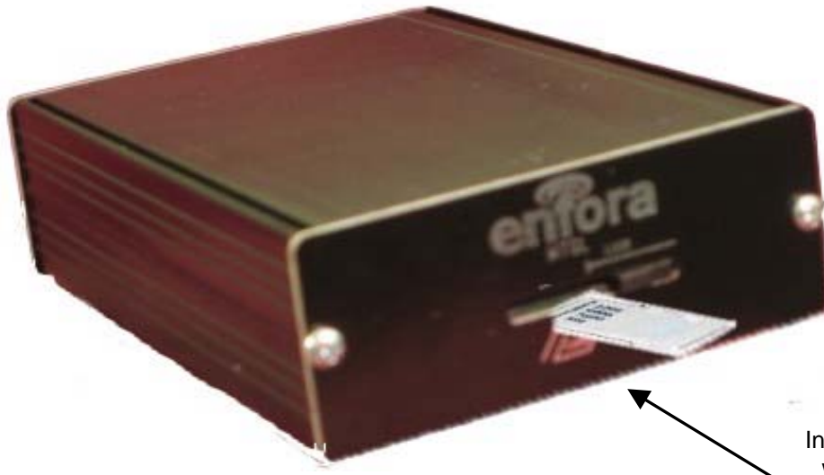
Figure 10 - Inserting a SIM
